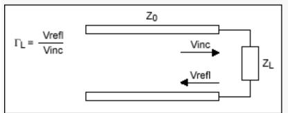
Figure 3. Impedance at the load.
