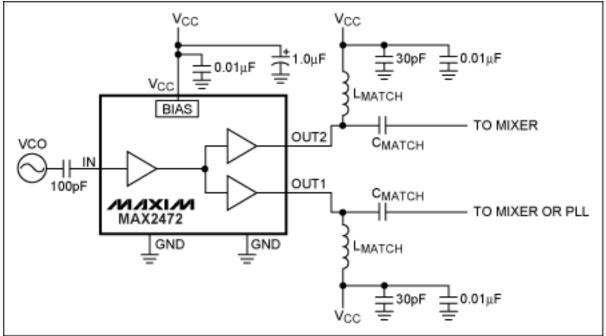
Figure 13. MAX2472 typical operating circuit.
