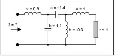
Figure 8. A multi-element circuit.
