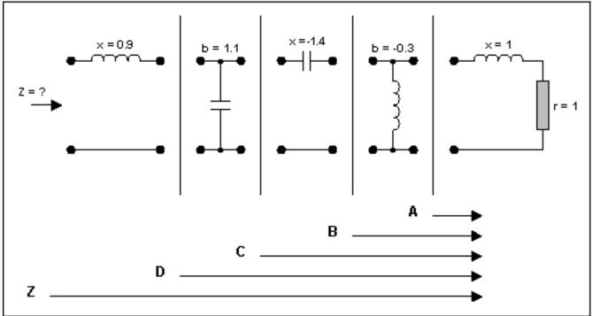
Figure 9. The network of Figure 8 with its elements broken out for analysis.
