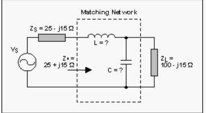
Figure 11. The representative circuit with known impedances and unknown components.
