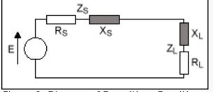
Figure 2. Diagram of  $R_S + jX_S = R_L - jX_L$ .
