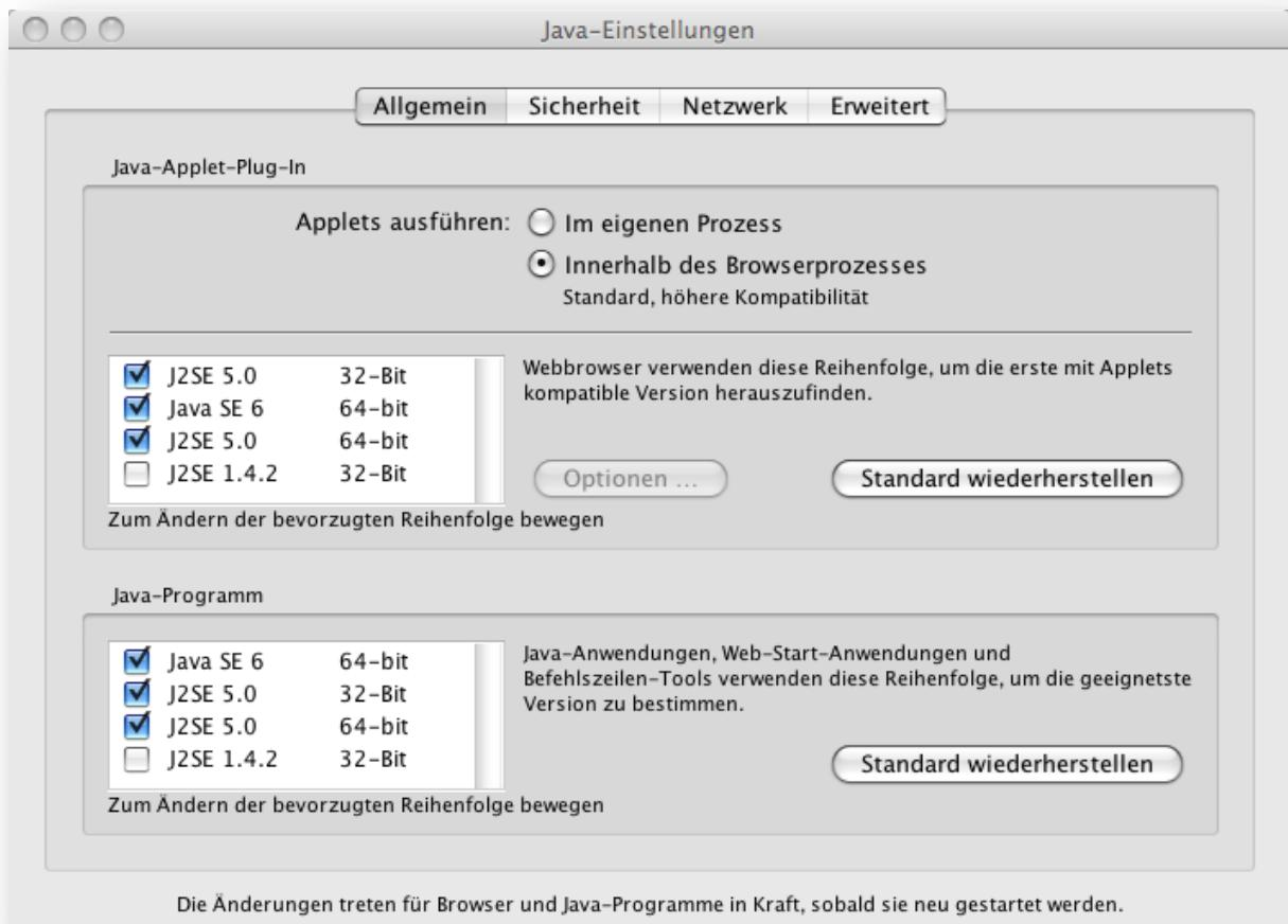
In the lower list (Java-Application) ensure, that at least a JAVA 5 version is available (means checkmark set) and that this version 5 is used prior to the 1.4 version.
