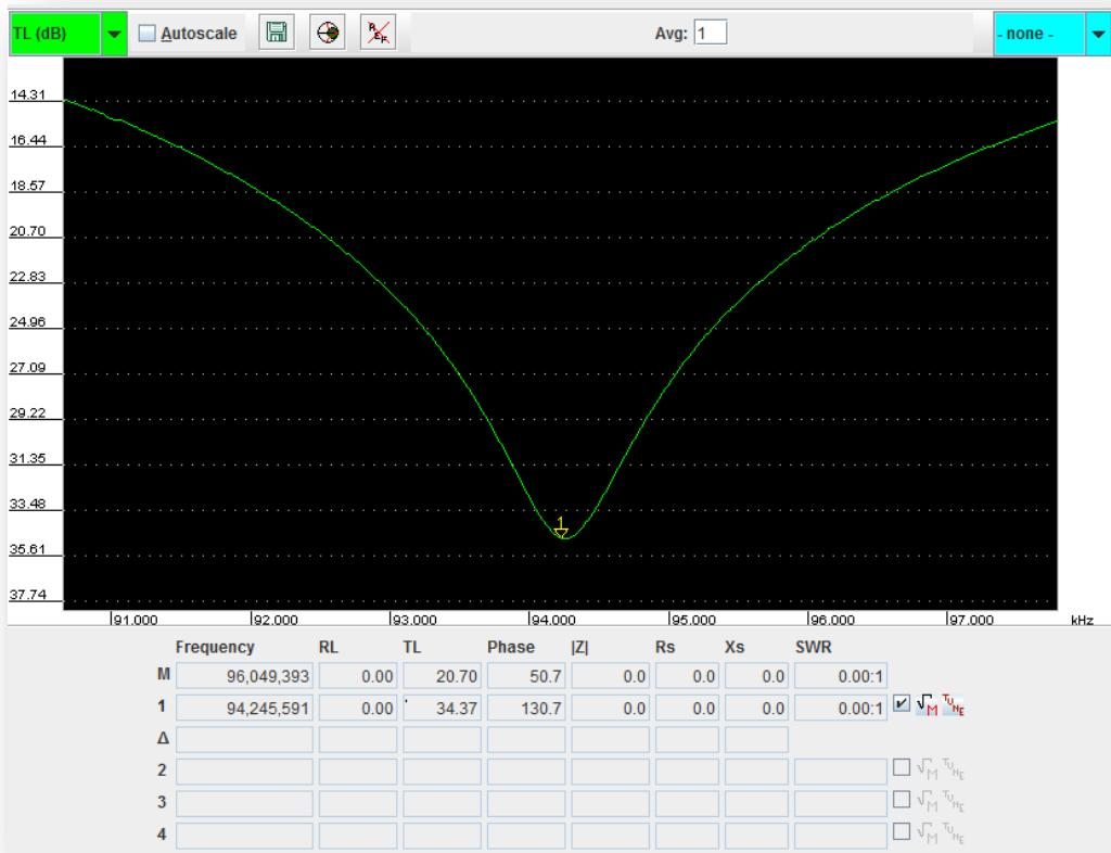
and cursor 1 should be set to the maximum transmission loss, here about 34dB at 94.2 MHz. The marker-math dialog should display these values:
