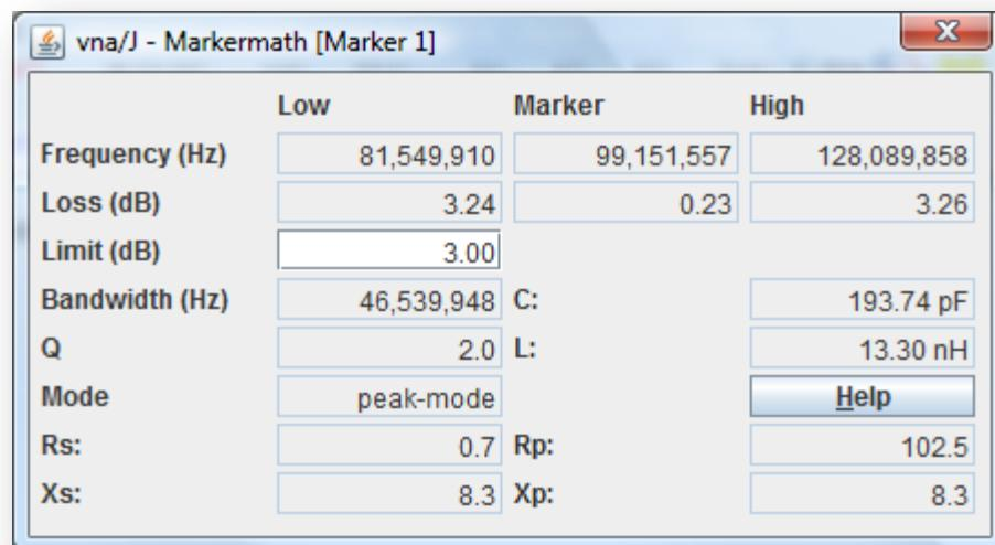
When I enter now the values for  $C=193,74\text{pF}$  and  $L=13,3\text{nH}$  I get this simulation inside RFSim99:
