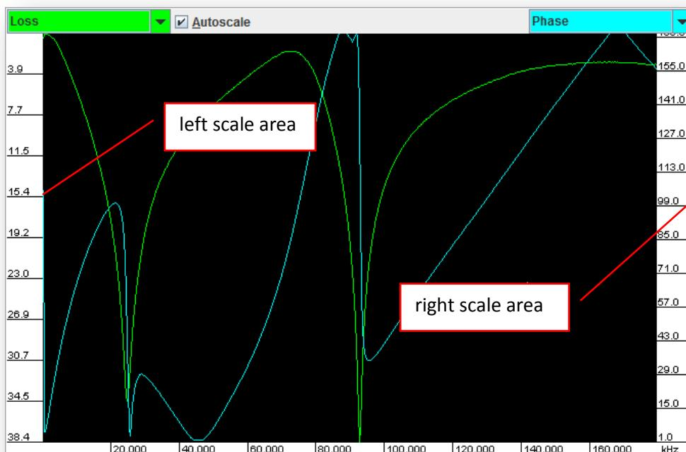
Clicking with the left mouse button on the scale area opens a small dialog, in which the user can enter the minimum (value at top of scale) and the maximum (value at bottom of scale):
