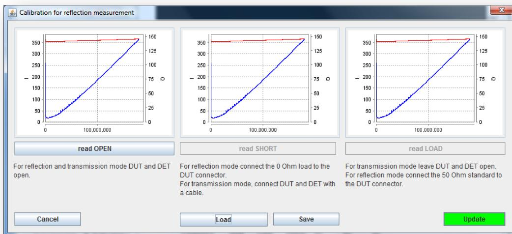
The calibration points are recalculated based on the current formulas implemented in the application to ensure also correct loading after update to internal mathematics...
