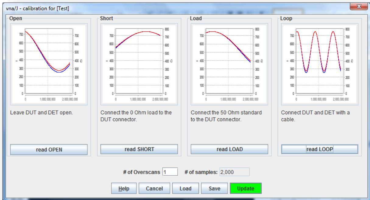
The created main calibration dataset can now be used in the application by simply pressing the UPDATE button, which will also close the dialog..
