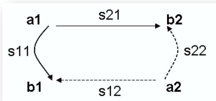
Currently the miniVNA is only capable of measuring the parameter S11 in reflection mode and S21 in transmission mode. The other parameters can only be measured, when manually reversing the DUT/DET connectors.
