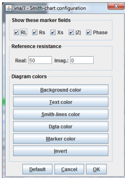
Here the data shown for each marker in the smith-chart can be configured. The marker-name and -frequency is always printed.
