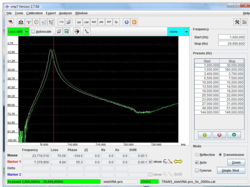
Only the left scale value is drawn from the reference data. The selected phase on the right scale is only drawn from the measurement data.
