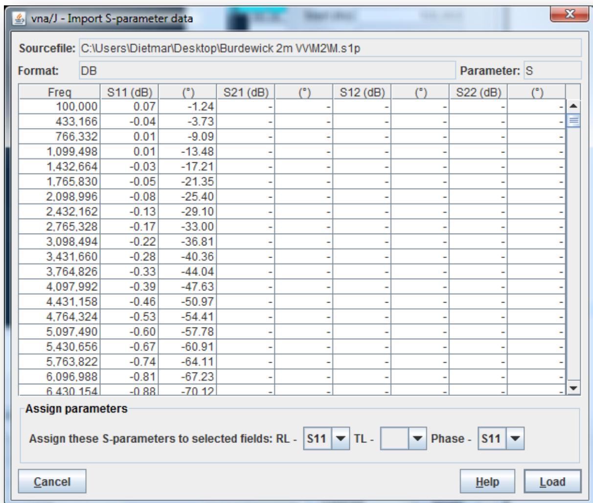
Here you have to choose, which data from the input file should be mapped to which data parameter inside vna/J.
