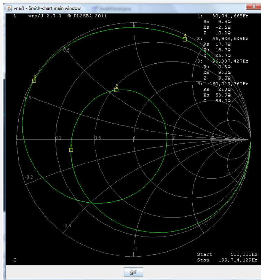
If the markers are selected in the main window, a small rectangle in the marker colour is drawn on the smith-chart and the configured marker data is printed on the right diagram side.
