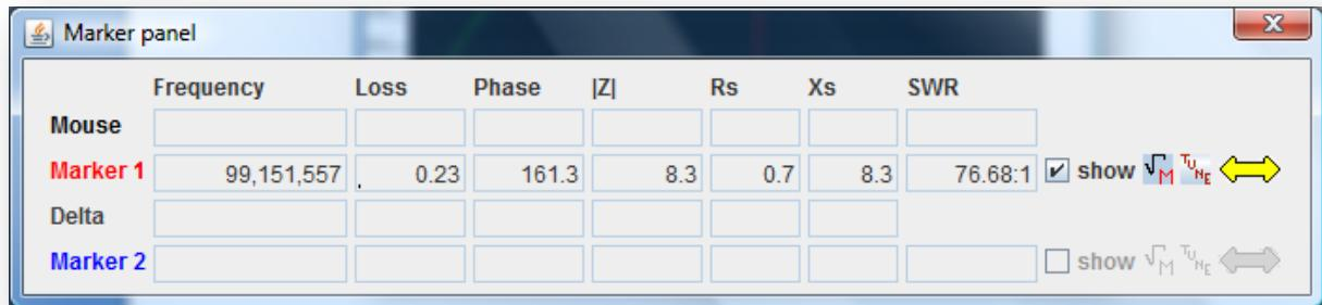
it automatically sets cursor 1 to 99.15 MHz - the minimum loss.
