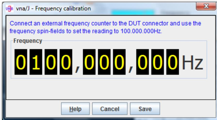
2. Connect a frequency counter to the DUT connector of the analyser.
