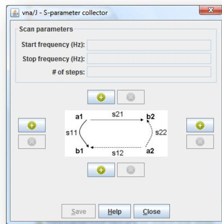
When you've executed a scan, you can put it into the collector by selecting one of the add-buttons
