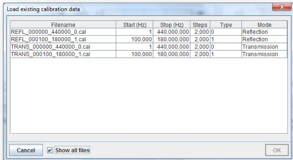
When the selected entry matches the current configuration (mode, frequency range, analyser type) the OK button is enabled.
