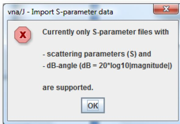
Please try to provide an S-parameter file with different format and parameters.
