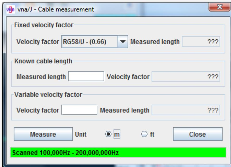
Pressing the MEASURE button starts a full scale scan of the attached analyser in reflection mode.
