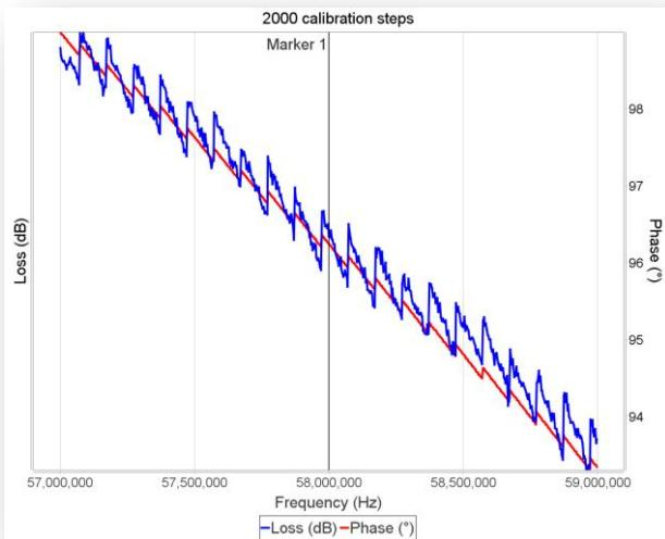
If the number of calibration steps is increased to 20.000 steps. This gives a frequency span of about 10kHz per calibration step. Now the same range is covered by 200 calibrations points. This results in a far more smooth measurement curve.
