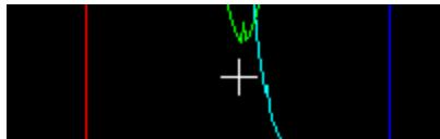
When the mouse is positioned inside the diagram panel, the current values at the mouse position are displayed in the marker named **M**.
