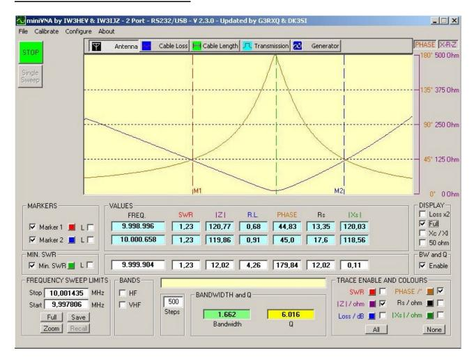
Connect the XTAL to the DUT connector and find at what frequency it has the lowest impedance.
