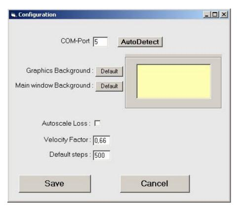
Use <u>Auto Detect</u> to identify and save the virtual Com-Port for the USB connection. If you want different Graphic or Background colours, click on the appropriate part of the frame and make your colour selection.
