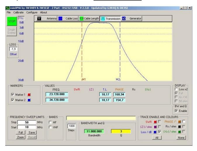
Connect the filter between DUT and DET. If it has an Insertion Loss you can compensate it in the <u>Loss Offset</u> box. To view the 3/6/10dB Bandwidth, just set both markers and enable the BW&Q.
