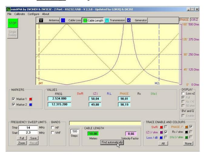
Connect the unknown cable to the DUT connector, then click the "Find Automatically" button.
