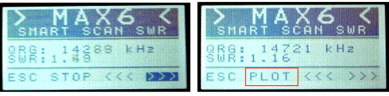
After finding the minimum SWR meter stops himself and appears key PLOT
