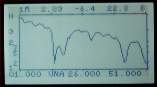
This allows us to measure the SWR of the antenna in any of our amateur band in a few seconds.
