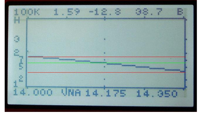
You can see that my GP antenna for 14 MHz band is in the middle of a SWR 1:1,59 38.7 ohm impedance. At the beginning of the band is about about the SWR 1:1.8 and end a band SWR 1:1.3
