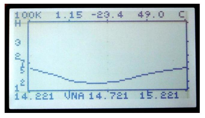
After pressing the **PLOT** graph appears SWR screen always displays measuring a width of 1 MHz and 100 kHz tuning step
